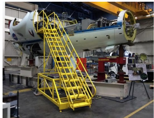
Figure 1: A mobile ladder stand platform used at a NASA facility. Source: www.wildeck.com/
